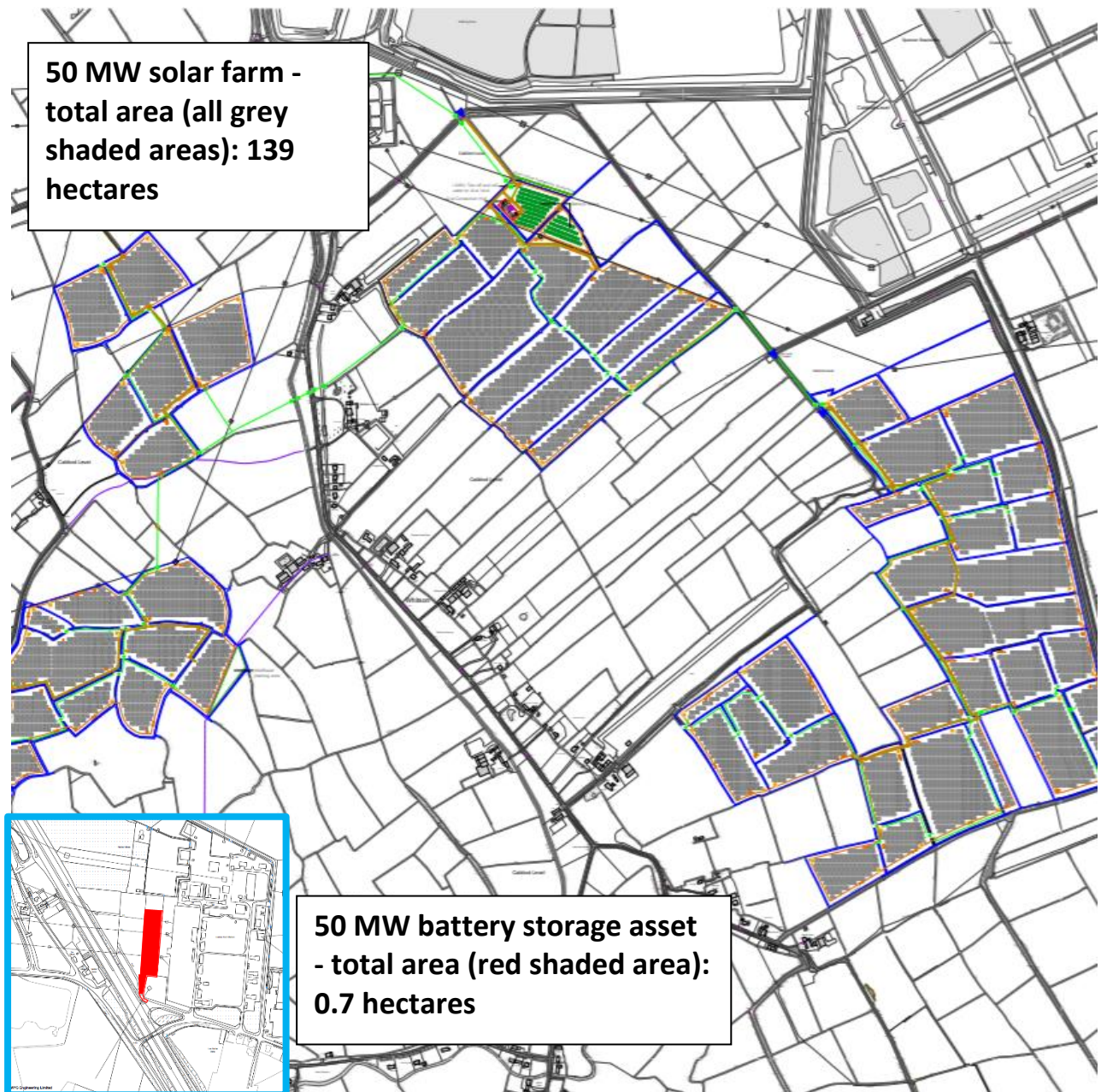
Fig 1. Size comparison between Gwent Farmers' Community Solar Scheme, 50 MW, South Wales 4 and Pivot Power, 50 MW battery storage, Carlisle 5
