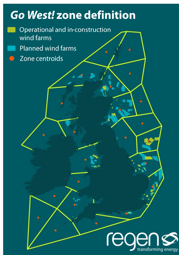
Figure 1: Zones used to model a variety of distributions of a 70 GW offshore wind fleet.
