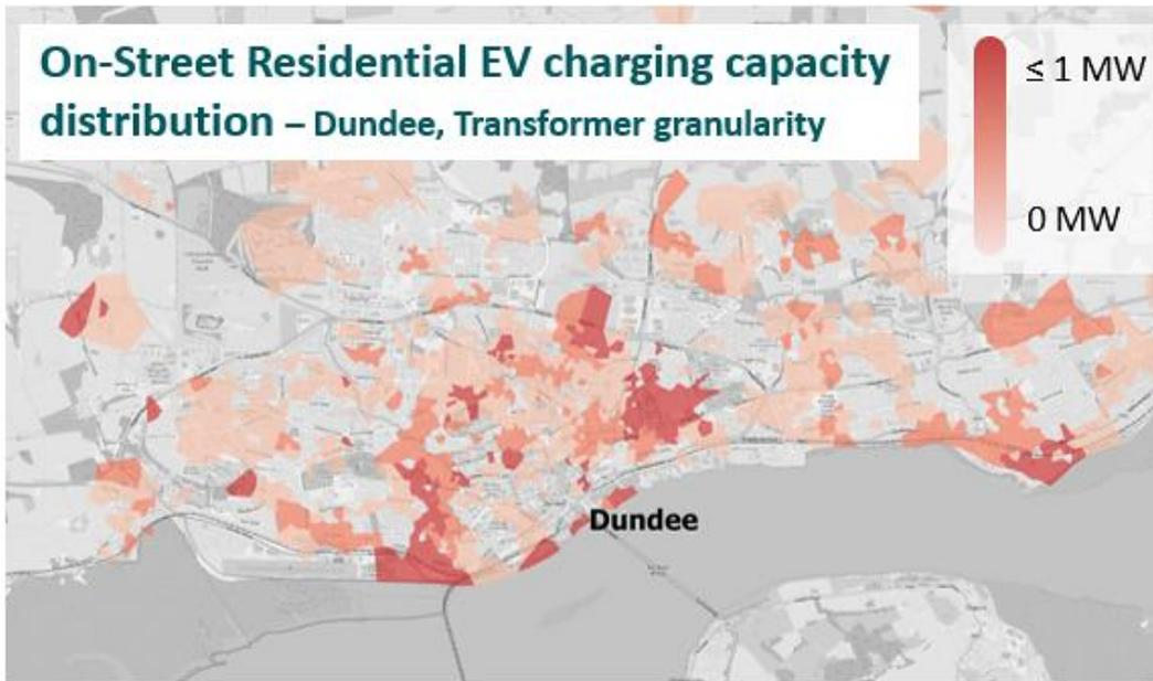
Figure 8: Transformer level geographic distribution of on-street residential EV charger capacity (MW) in Dundee in 2050, under the **Consumer Transformation** scenario
