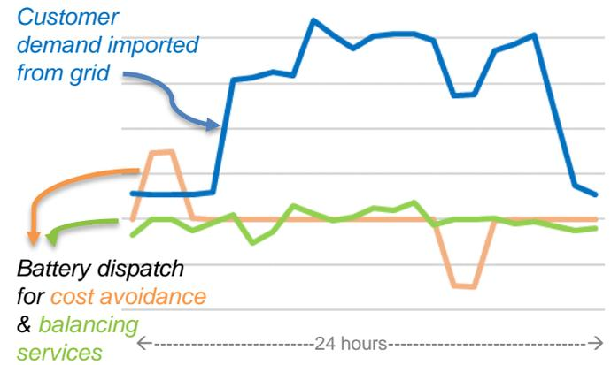
**Balancing services income:** The storage system can be configured to generate revenues from supplying services to National Grid, for example by reducing or increasing electricity usage at the site. The business is paid for this service, but uses the battery to flex site load rather than adjusting its actual electricity demand
